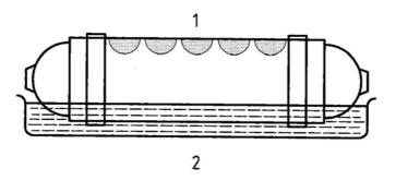
Then the cylinders are pressure cycled between 20 bar and 260 bar for up to 1 000 times per year of design life, at ambient temperature, high temperature (82 °C) and low temperature conditions (-35 °C).
